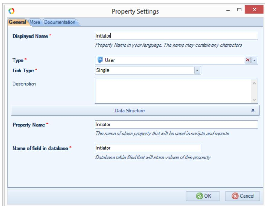
Fig. 53 Configuring property settings of the process variable
