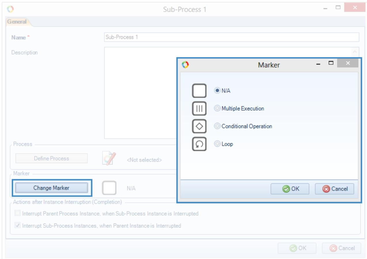
Fig. 126. The Change Marker button and the marker selection window
