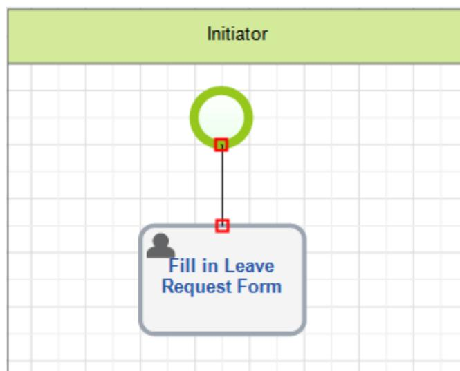
Fig. 63. Adding a flow line
