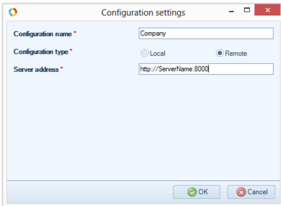
Fig. 17. Adding a remote configuration
