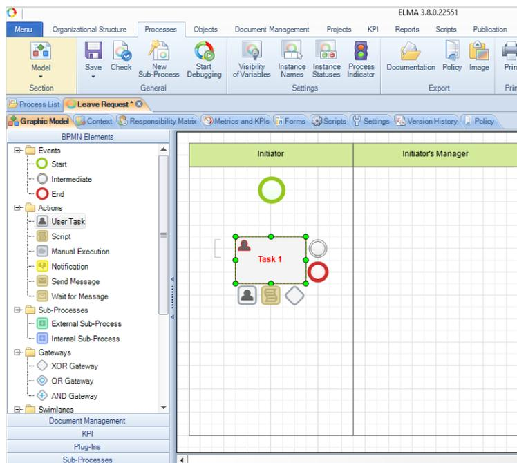
Fig. 58. Adding a User Task element
