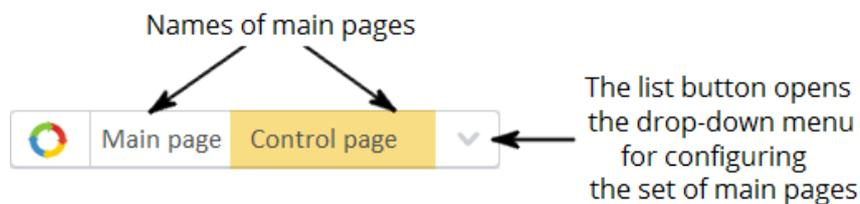
Fig. 19. Drop-down menu for configuring the set of main page
